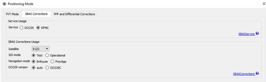
**Figure 1 – Receiver configuration window showing the selection of the SBAS stream used in Canberra**
