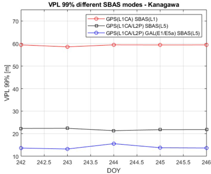
Figure 12 –P99 Vertical Protection Level Performance at Kanagawa.
