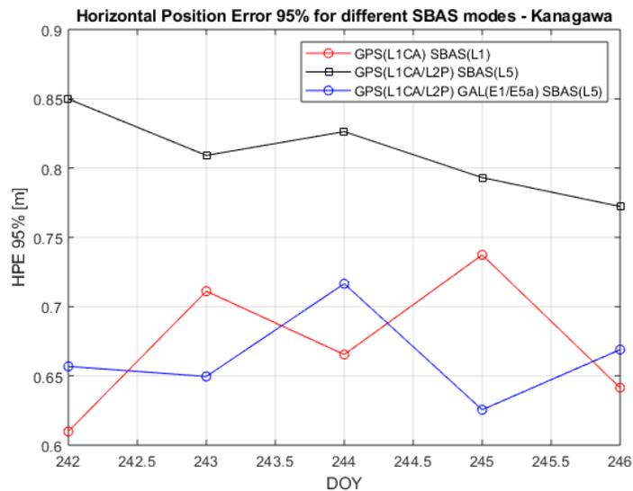
**Figure 10 – Horizontal error P95 performances for the receiver in Kanagawa**
