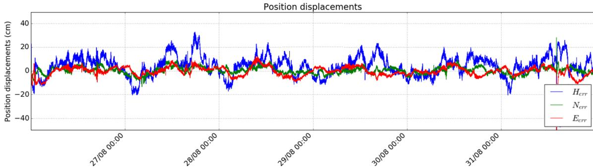
Figure 13 – PPP Position with Testbed GPS+GAL RTCM corrections
