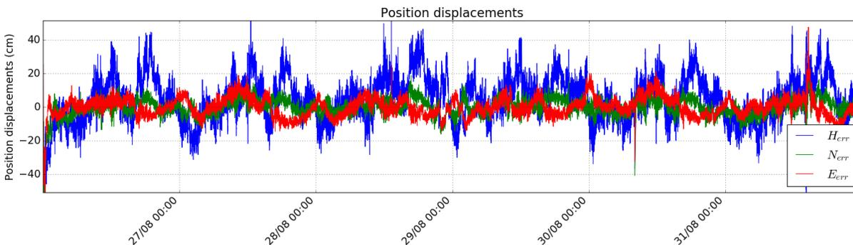
Figure 14 – PPP Position with Testbed GPS SBAS L1 corrections
