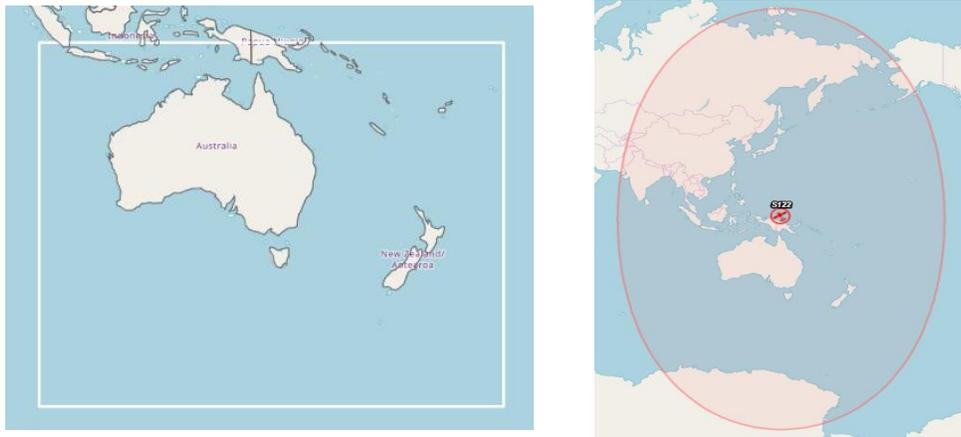
Figure 4 – SBAS L1 (left) and SBAS L5 (right) coverage areas
