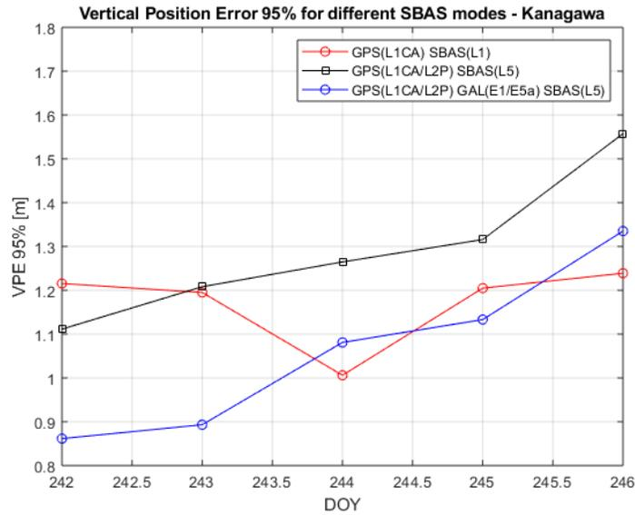
**Figure 11 – Vertical error P95 performances for the receiver in Kanagawa**
