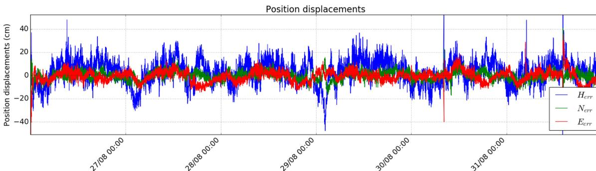
Figure 15 – PPP Position with Testbed GPS+GAL SBAS L5 corrections
