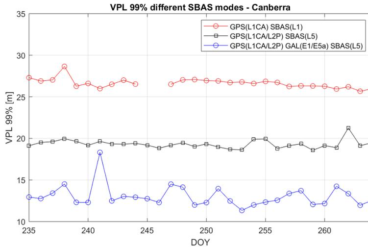
Figure 8 – P99 performance of Vertical Protection Level at Canberra.
