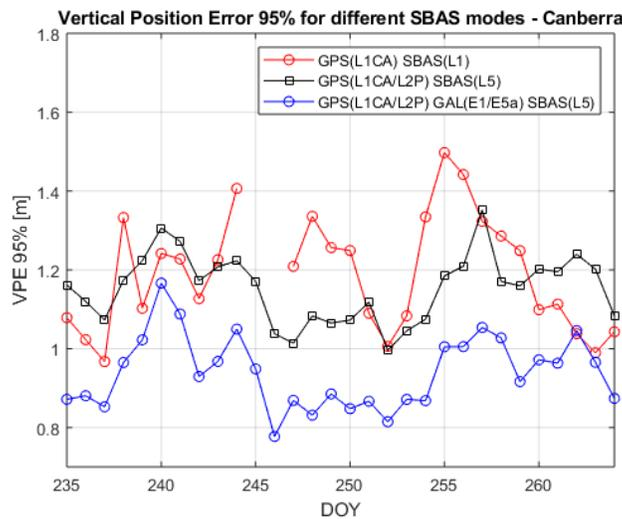
**Figure 7 –Vertical Error (in terms of P95 performance) at Canberra receiver**
