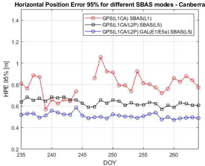
**Figure 6 – Horizontal errors (in terms of P95 performance) at Canberra receiver**
